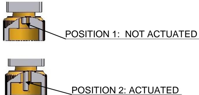
Before threading the electrical actuator to the activation port of the valve, check that the actuator pointer is retracted (position 1).
